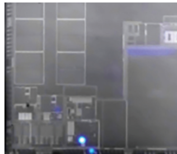
Photoemission microscopy on IC using water cooled SWIR InGaAs camera, with 20x objective, exposure time 30s
