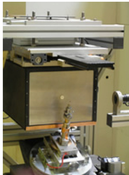
Fig. 2. OrientExpress: the new Laue diffractometer.
